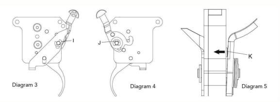
The TacSport Pro is shipped with a safety lever and a bolt stop release lever. The bolt stop and safety can be removed. They are kept in place by a small e-clip which can be removed by spreading the legs of the clip with a screwdriver I and J in diagrams 3 and 4. Please keep the spring washer and a ball-bearing that come with the safety lever and bolt stop.
